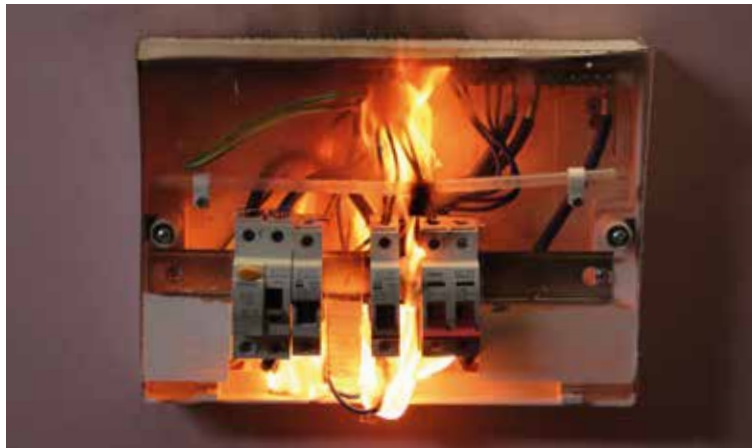
Fire in the consumer unit just before tube bursting
