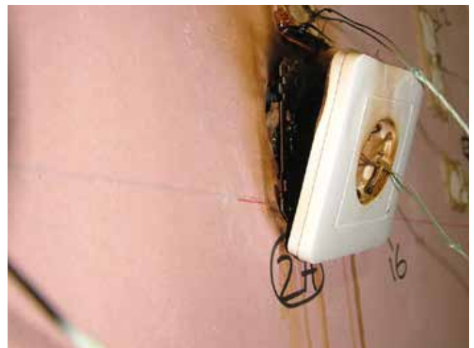
Protected socket after 90 minute test
