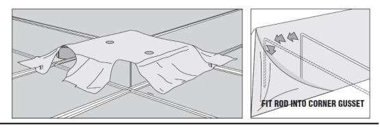
2. With the tent laid out, turn it to its upright position and insert rod ends into their pockets placed at each corner of the tent.
