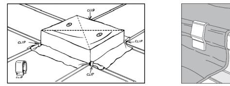
3. Place the tent over the light fitting and fit the cable through the ventilation hole and connect to the light fitting according to the manufacturer's instructions. Go to each corner and pull the material away from the fitting over the T-bar and fix the material to the T-bar with the clips supplied. Pinch each clip with a pair of pliers to fix tightly.
