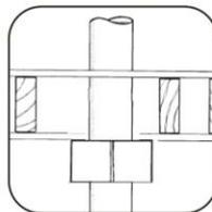
Surface-mounted into hollow timber floors.
